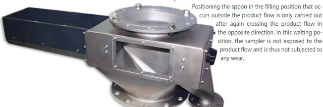
curs outside the product flow is only carried out after again crossing the product flow in the opposite direction. In this waiting position, the sampler is not exposed to the product flow and is thus not subjected to any wear.
