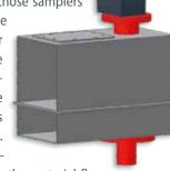
ple collecting pipe protruding in the material flow that is provided with openings. Normally, these openings are turned in the direction of conveyance and close against a sealing gasket. At the time of sampling, the sample collecting pipe with its openings is turned against the direction of conveyance, so that sampling material can flow in. The sample material thus entered is discharged downwards through the air slide conveyor system by means of the sample collecting pipe.
