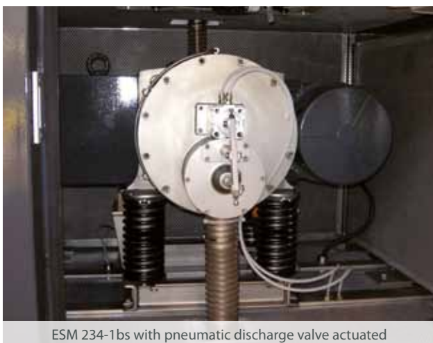
sound isolation cover with feeding and discharge equipment
