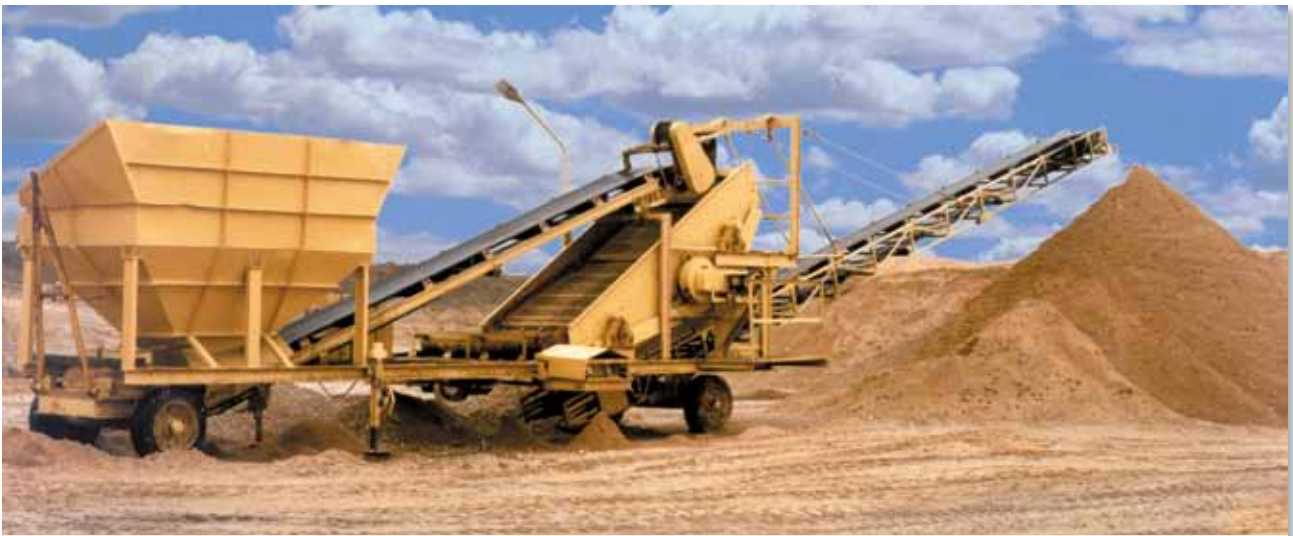
Mobile sand screening plant consisting of circular motion screening machine, feed hopper, belts and chassis.
