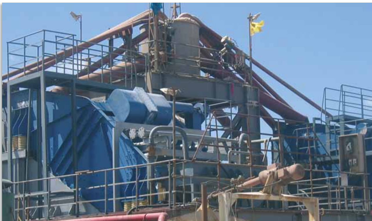
Double counterweight banana screen for dewatering in a potash mine
