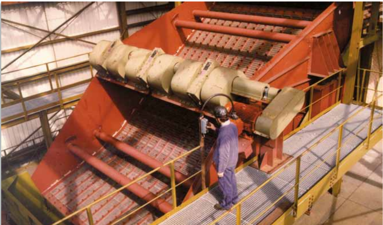
Double counterweight screen BHG, for pre-classifying raw washed coal
