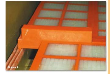
**Picture 1** shows an adjustable back wall with removable ribs combined with screen segments.
