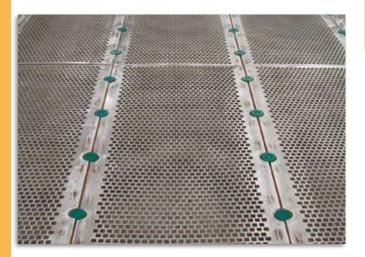
Hybrid segments are an ideal combination between highly wear resistant polyurethane and steel screen segments of various types.
