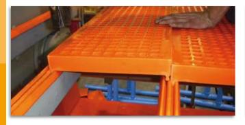
**UNI 2000 - system screen modules** are fixed to the substructure bars by means of adapter slats, thus making it compatible to other types of modular systems. There are system units with standard widths of 150 and 300 mm and flexible lengths of up to 1200 mm, all made of highly wear resistant polyurethane.
