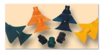
**Aquaplast-Fan Spray Nozzles**, of corrosion and wear resistant polyurethane, virtually eliminates blockages even with particles up to 3 mm in the water. Well proven for washing / rinsing on screening machines, with an even, fan shaped water curtain using pressures of 0,5 to 3,5 bar.
