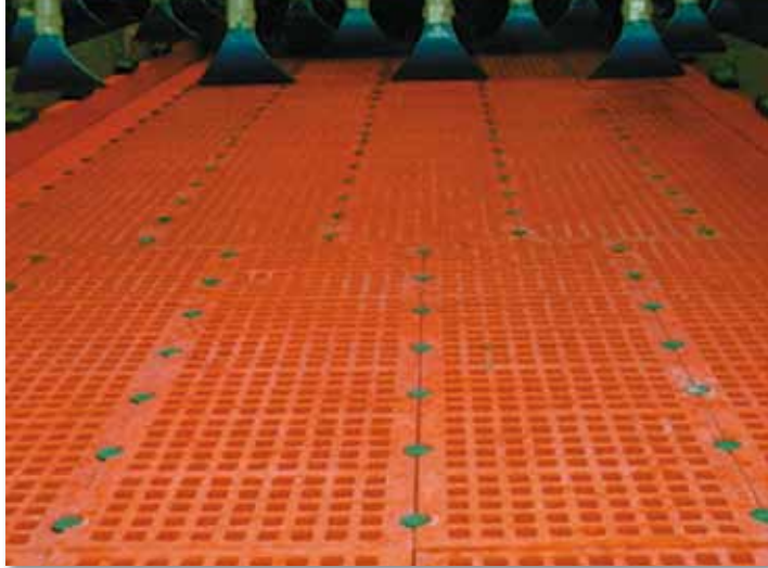
Sieve panels of highly wear resistant polyurethane... in modular, tensioned or flat panel designs for the separation of bulk materials such as sand and gravel, hard rock, coal and ore, chemical products, foodstuffs and many other materials.
